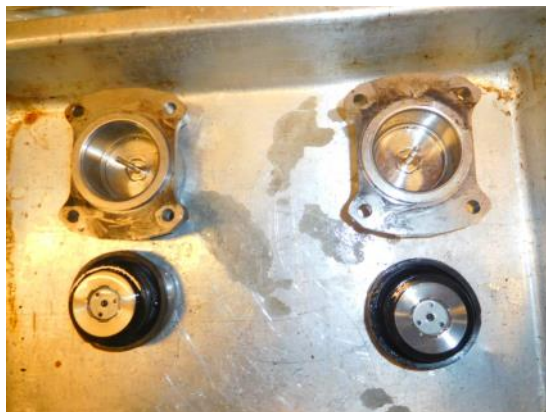
Passenger's side Rear HYE-DRA-CYL Stainless Steel Cylinder condition
