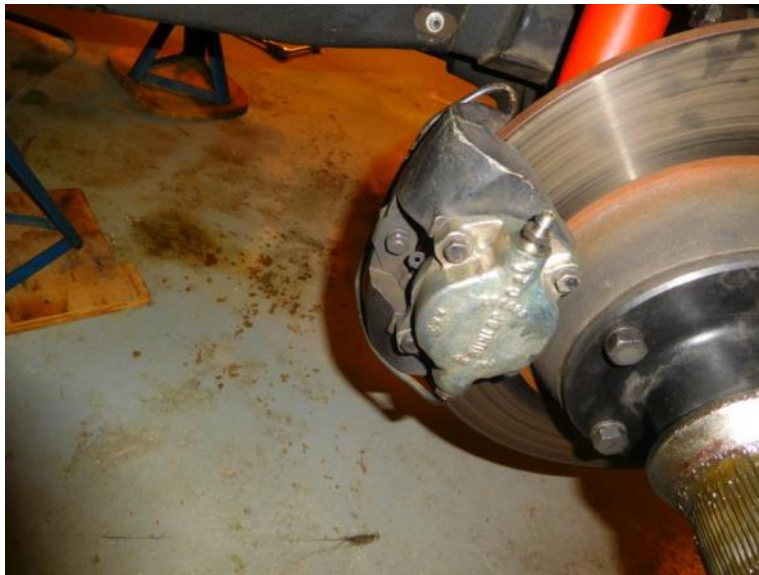
Typical, twin cylinder square puck Series 1 Dunlop Disk Brakes.
