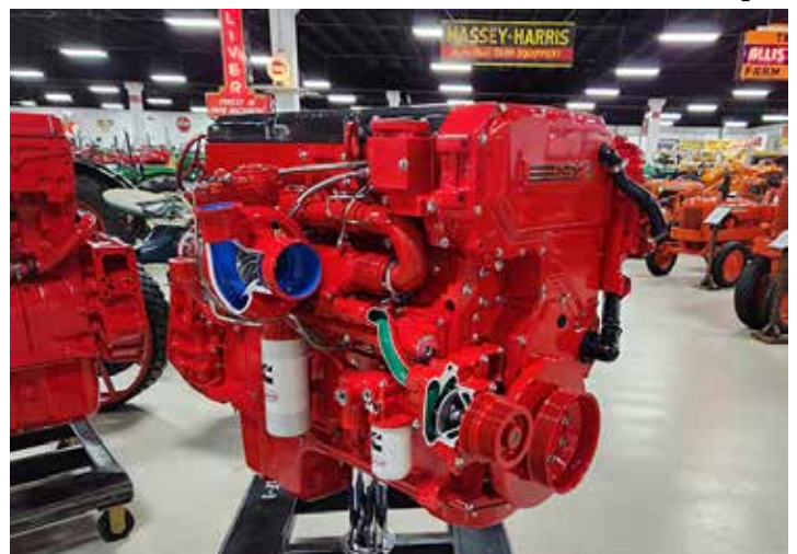
As a retired Service and Customer Support Manager for Cummins High Horsepower Engines, Brian Trickett homed right in on this Cummins ISX.
