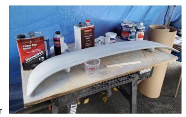
lems that result if you don't. He talked about experimenting with fan pattern adjustments on cardboard before moving to the car, finding the Goldilocks application rate to avoid runs and dry or orange-peel areas, and more.
