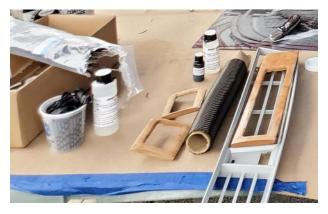
Randy then moved to the table with carbon fiber elements. He had a few old wood interior Jaguar parts that he said could be wrapped in carbon fiber for a contemporary look (*left*). The woven carbon fabric can be cut with very sharp scissors and molded around compound curves using resins as the matrix.
