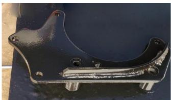
coating. Using an engine accessory bracket brought by Brian Case, they first media blasted it in an inexpensive
